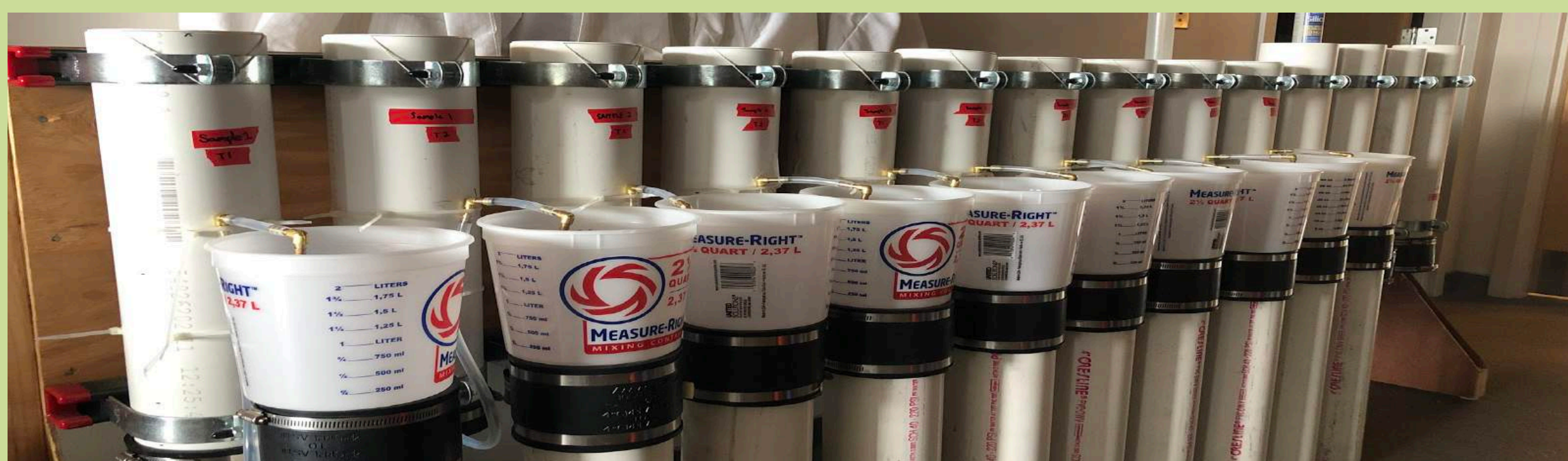
Figure 2, Pilot scale sand columns and effluent water collection system
